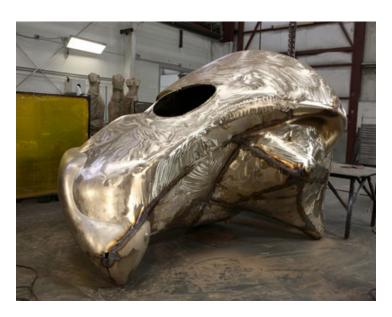
Here, we used state-of-the art imaging and modeling, and then went into a traditional foundry in Walla Walla [Washington] where they took the digital files and built the molds out of plaster-impregnated foam. We were able to bypass building the whole sculpture out of clay step, like any sculpture in the 20th century is made. I think it was fun for Jason and Steve to see something come back that was 20,000 pounds of bronze, when they were so used to computing in this scaleless, airless space.
